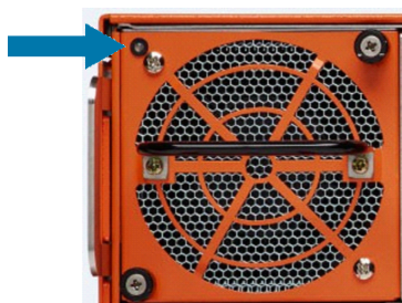
Figure 6 Individual Fan LED Location on GigaVUE-HC3 Rear
